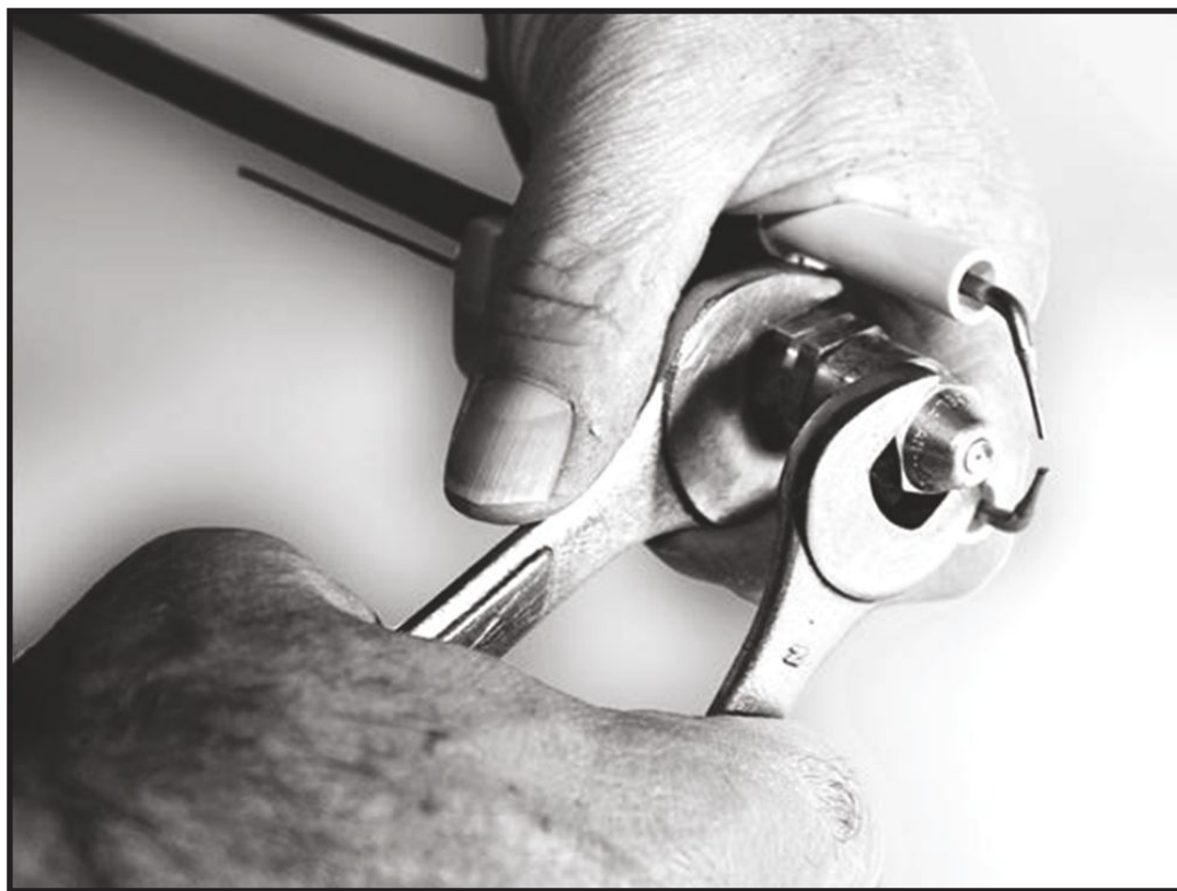
Figure 3G : CAREFULLY SUPPORT THE NOZZLE ADAPTER WHEN REMOVING OR INSTALLING NOZZLE
